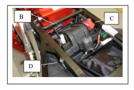
**STEP #4** -The center terminal is plus and the outer ring is negative (see dwg below). Apply either dielectric grease or Vaseline to terminals. Connect the red wire to the POSITIVE terminal and the black wire to the NEGATIVE terminal. Use a voltmeter to check if the polarity is correct.
